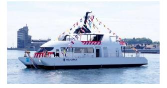
*Fig.* 11: *Hydrogen/bio-fuelled ship "HANARIA"* (Source: <u>https://www.mol.co.jp/en/pr/2023/23111.html</u>)
